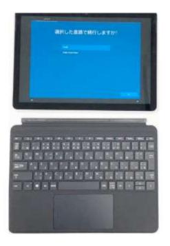
Connect the Surface device to the keyboard in the direction shown in the picture.
